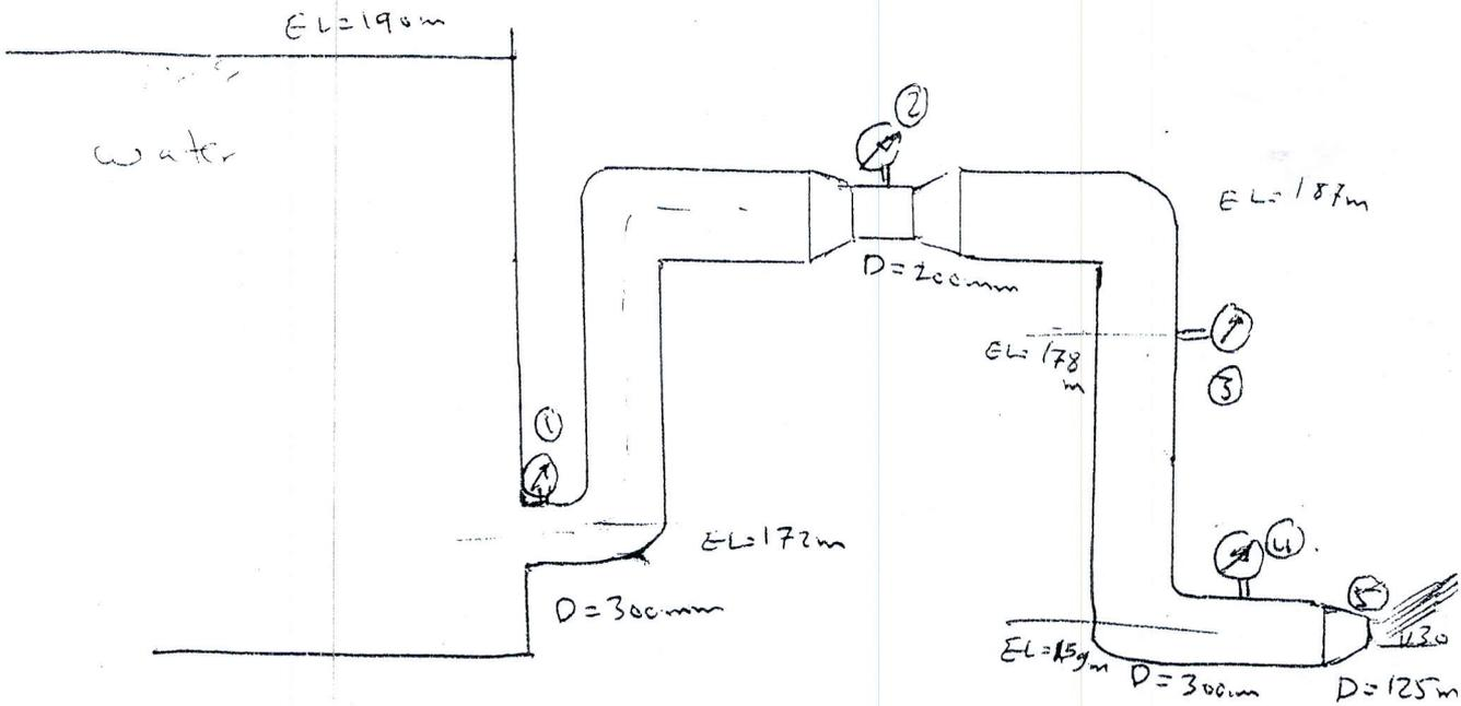
Ex 14) Evaluate the discharge through the system shown & the pressure in each shown point, Draw the energy line & Hydraulic gradient line.
