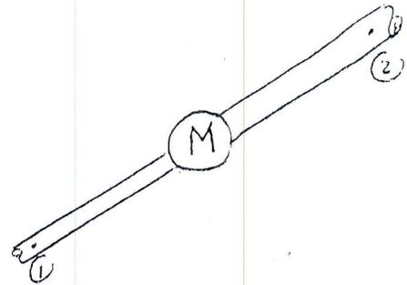
For the figure above (M) represent any machine installed in the pipe system shown. Bernoulli's equation between 1 + 2 with existence of (M) may be written as follow:-
