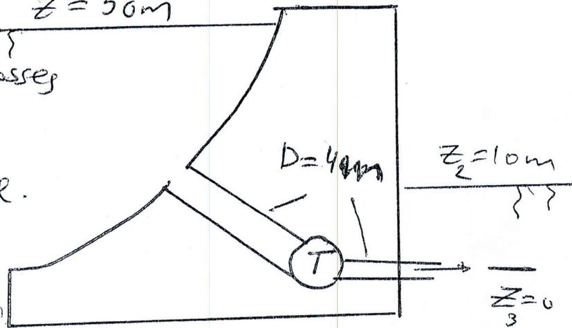
$$\frac{P_1}{\rho} + \frac{v_1^2}{2g} + z_1 = \frac{P_2}{\rho} + \frac{v_2^2}{2g} + z_2 + h_f + h_T$$
