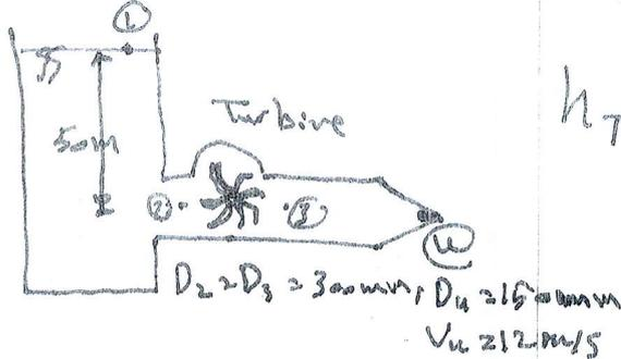
$$\frac{P_1}{\rho} + \frac{V_1^2}{2g} + z_1 - h_T = \frac{P_4}{\rho} + \frac{V_4^2}{2g} + z_4$$
