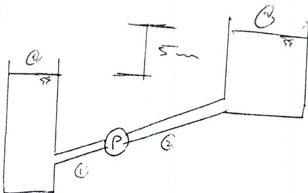
Evaluate the discharge when the pump gives a head of (20m). Assume the losses in the first line is  $(h_{L1} = 5 \frac{V_1^2}{2g})$  the diameter of first line is (150mm). the losses in the second line  $(h_{L2} = 12 \frac{V_2^2}{2g})$  and its diameter is 100mm. take  $\alpha = 1$  for two pipes. what will be the horse power of the pump.
